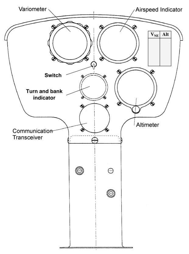
Instrument Panel in Forward Cockpit Fig. 7.3
