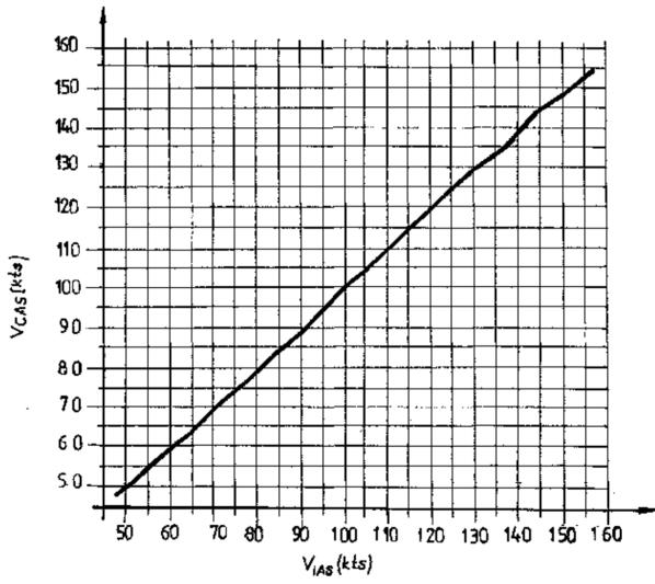
Airspeed Indicator System Calibration Fig. 5-1
